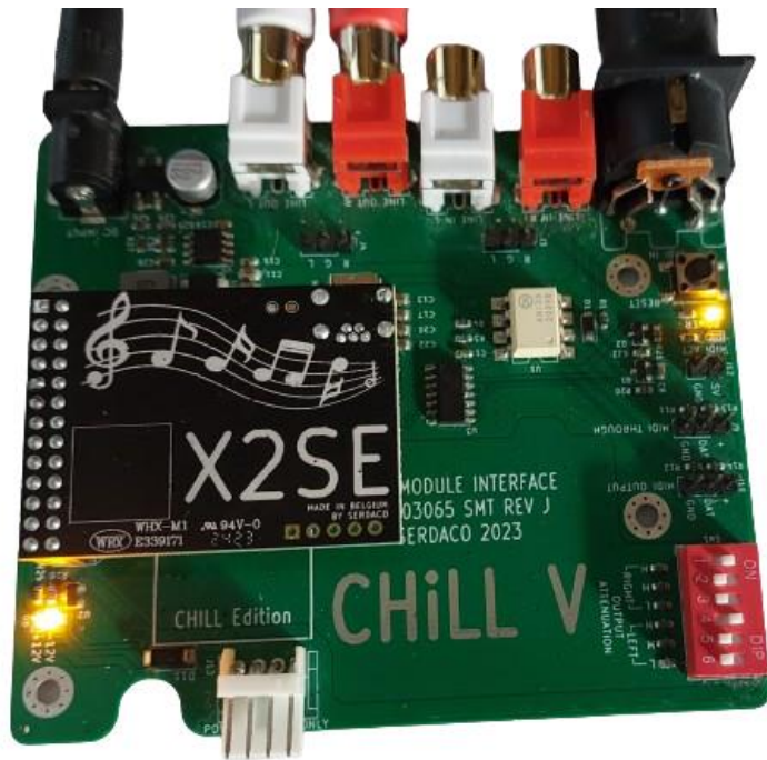
Figure 28: X2 mounted on CHiLL interface
