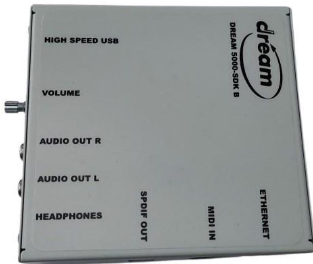
Figure 2: Dream 5000 SDK hardware module
